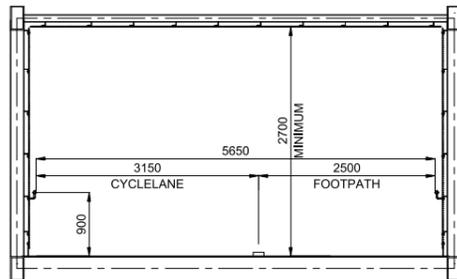
TYPICAL SECTION THROUGH CENTRAL SPAN
