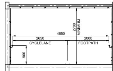
TYPICAL SECTION THROUGH ARTERIAL LINK SPAN
