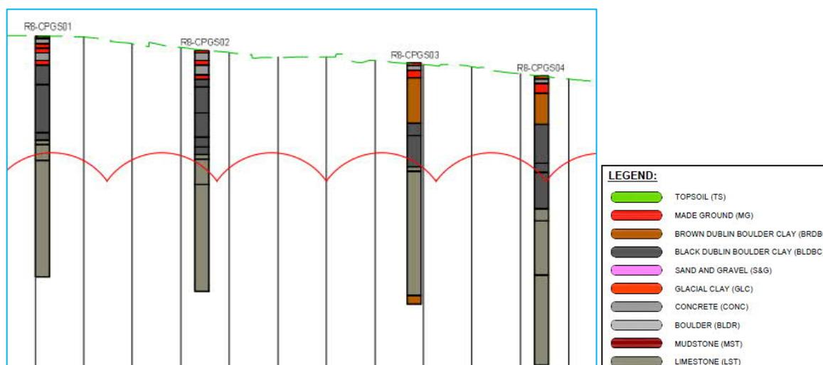
Figure 2.3 Geotechnical Longitudinal section
